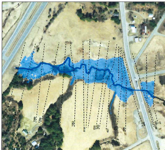
Base flood inundation extent at Newbury Leighton Hill Solar site determined using 1D HEC-RAS model.
