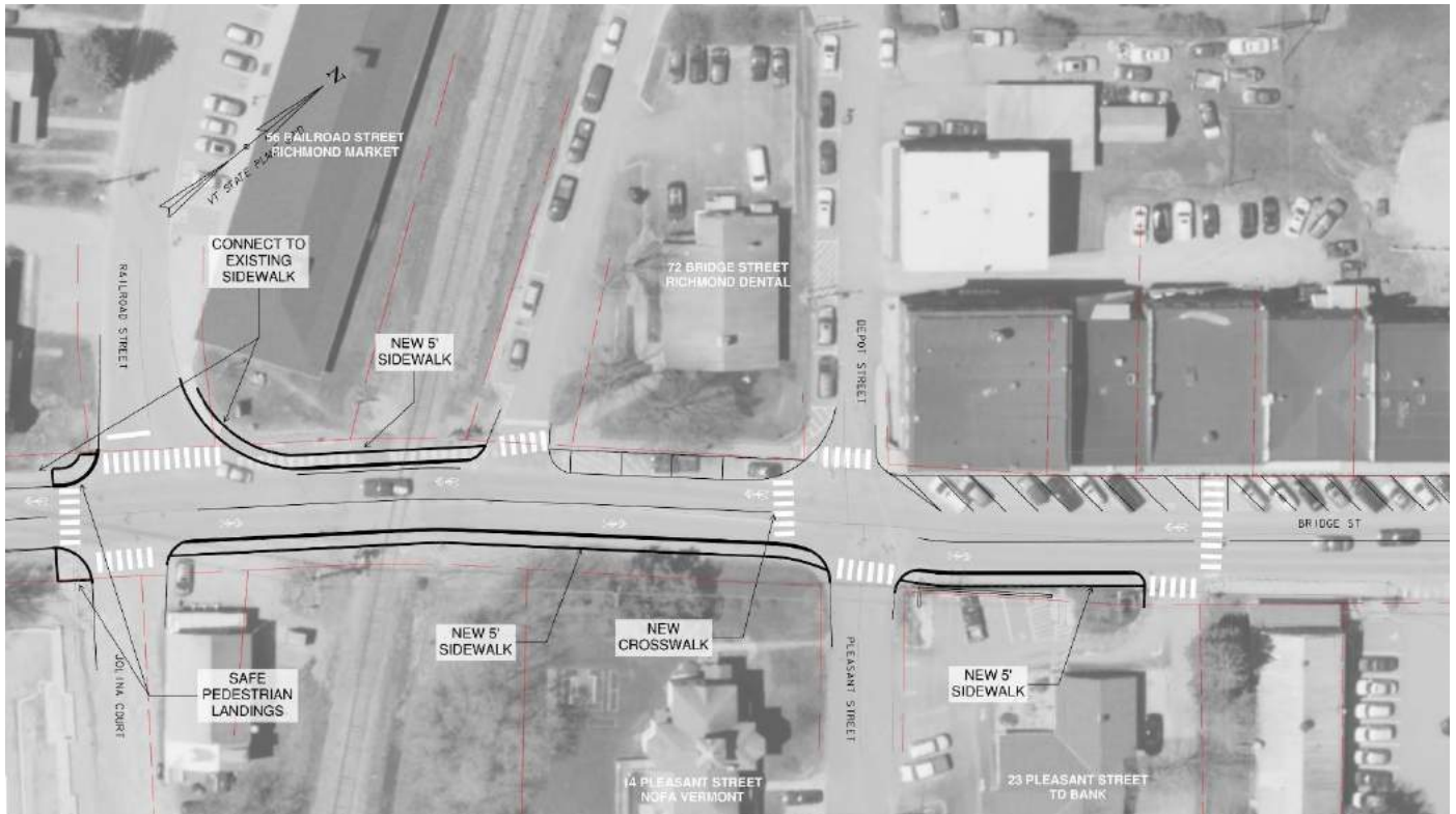
Figure 1. Alternative 1 – Sidewalk and Shared Lanes
