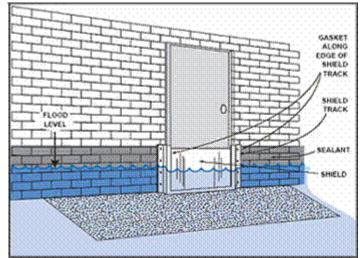
Figure 6.8-4. Example of a dry flood proofed commercial building.
