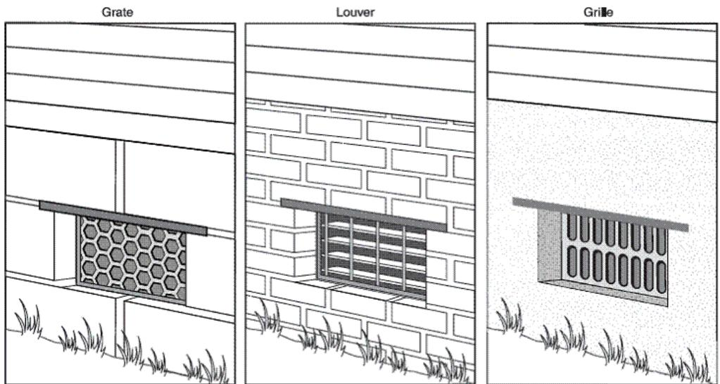
Figure 6.8.4 - Example of an elevated structure on a wet flood proofed, at-grade crawl space with an opening which permits the automatic entry and exit of floodwaters.
